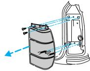
assembly off and to the right (it may be necessary to use a screwdriver to remove the lamp assembly).
